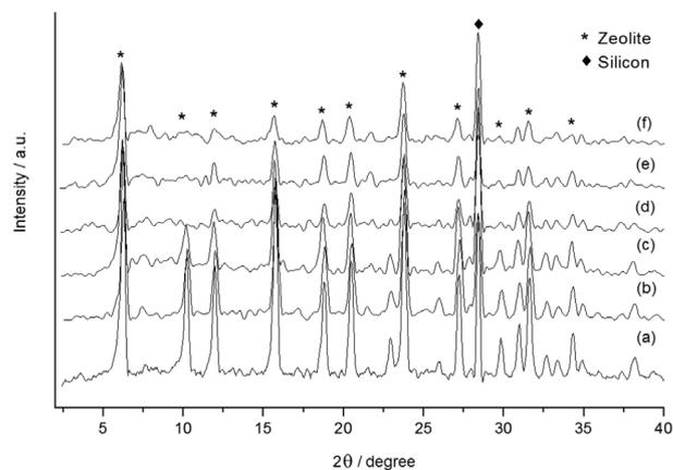
**Figure 2.** Diffractograms of HUSY (a) and Ce-USY catalysts calcined at 550 °C for 8 h containing 2 (b), 5 (c), 10 (d), 15 (e) and 25 wt.% of CeO<sub>2</sub> (f).
