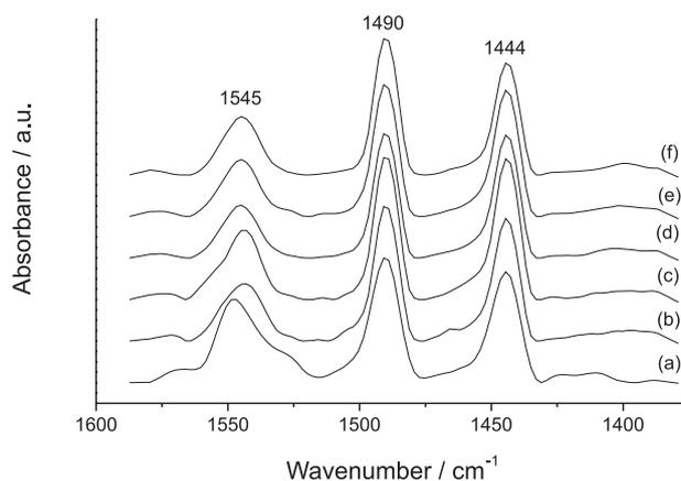
**Figure 8.** FTIR spectra of HUSY and Ce-USY (calcined at 550 °C for 8 h) after pyridine adsorption and thermal desorption at 150 °C: HUSY (a) and Ce-USY catalysts containing 2 (b), 5 (c), 10 (d), 15 (e) and 25% wt. of CeO<sub>2</sub> (f).
