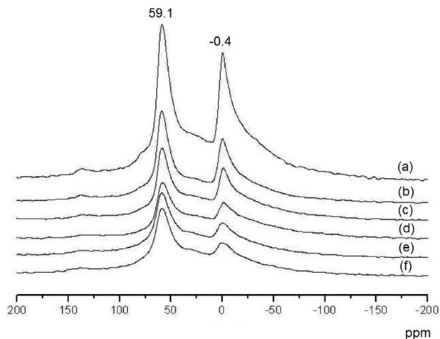
**Figure 5.** <sup>27</sup>Al MAS NMR spectra of HUSY (a) and Ce-USY catalysts calcined at 550 °C for 8 h containing 2 (b), 5 (c), 10 (d), 15 (e) and 25% wt.% of CeO<sub>2</sub> (f).
