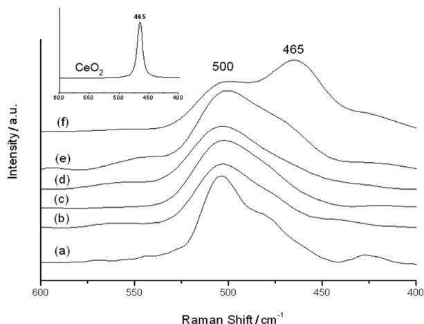
**Figure 4.** FT-Raman spectra of HUSY (a) and Ce-USY catalysts containing: 2 (b), 5 (c), 10 (d), 15 (e) and 25% wt.% of CeO<sub>2</sub> (f) calcined at 550 °C for 8 h. The spectrum of CeO<sub>2</sub> (inset) is also shown for comparison.
