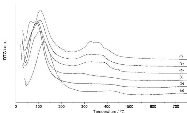
**Figure 1.** DTG curves, all before calcination, of HUSY (a) and Ce-USY catalysts containing 2 (b), 5 (c), 10 (d), 15 (e) and 25 wt.% of CeO<sub>2</sub> (f).
