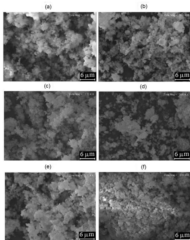
**Figure 7.** SEM micrographs of HUSY (a) and Ce-USY catalysts calcined at 550 °C for 8 h containing 2 (b), 5 (c), 10 (d), 15 (e) and 25% wt. of CeO<sub>2</sub> (f).
