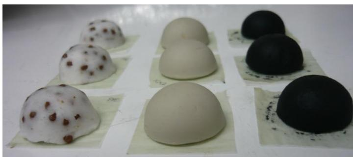
**Figure S2.** Monolithic dispensers for 3-pentanol made of paraffin oil (60%) + paraffin mp 53-57 °C (40%) with 20% activated charcoal (black color), 20% kaolin (grey color) and 20% molecular sieve (white and brown color).
