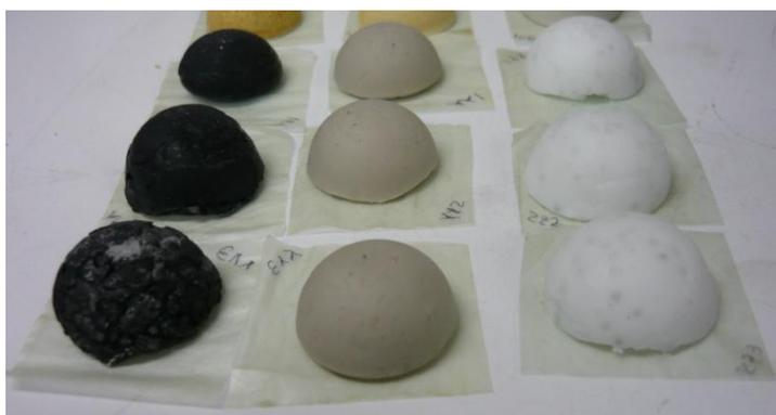
**Figure S1.** Monolithic dispensers for 3-pentanol made of paraffin oil (60%) + paraffin mp 53-57 °C (40%) with 20% glass spheres (white color), 20% activated charcoal (black color) and 30% kaolin (grey color).
