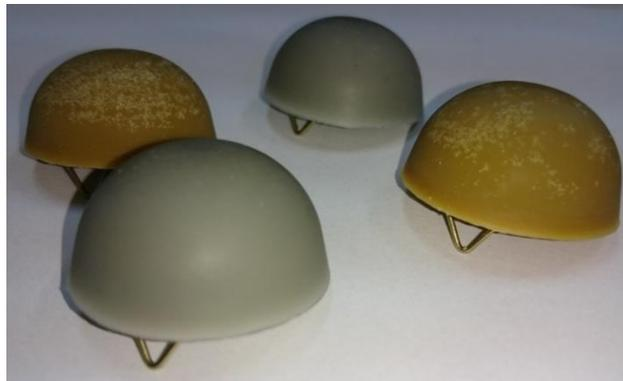
**Figure S4.** Dispensers used in the field trials. Monolithic dispensers for sulcatone made of paraffin oil 70-80 °C with 30% kaolin (grey color). Dispensers for sulcatol and 3-pentanol made of carnauba wax mixed with 30% kaolin (beige color). A hook was inserted in the dispensers for their placement in the trees.
