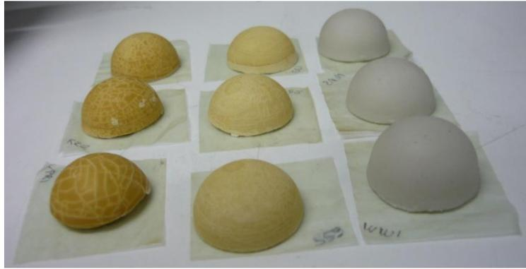
**Figure S3.** Monolithic dispensers for sulcatone made of paraffin oil (60%) + paraffin mp 53-57 °C (40%) with 10% kaolin (grey color) and with carnauba wax mixed with 20% kaolin (light beige color) and 30% kaolin (beige color).
