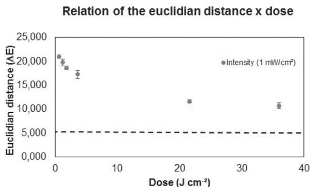
**Figure 3.** Euclidean distance ( $\Delta E$ ) as a function of delivered light dose (D) for cotton fabric samples treated with  $H_2O_2$  40% and UV light at  $1 \text{ mW cm}^{-2}$ . The dashed line at  $\Delta E = 5.3$  corresponds to the OBCF.
