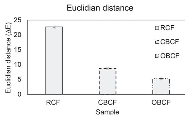
**Figure 2.** Euclidian distance (ΔE) between calibration white and raw cotton fabric (RCF), chemically bleached cotton fabric (CBCF); optically bleached cotton fabric (OBCF).
