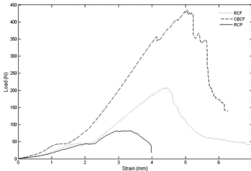
**Figure 4.** Tensile test in raw cotton with load as a function of strain. Raw cotton fabric (RCF) corresponds to the dotted line, chemically bleached cotton fabric (CBCF) corresponds to the dashed line and photobleached cotton fabric (RCP) corresponds to the continuous line.
