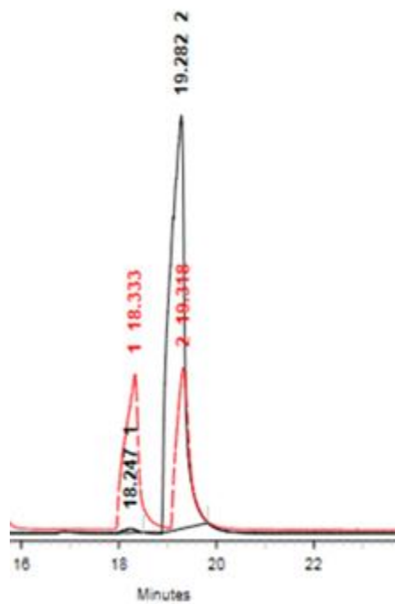
Figure S12. Chromatogram of racemic mixture 8 , superposed to the chromatogram of 12 .
