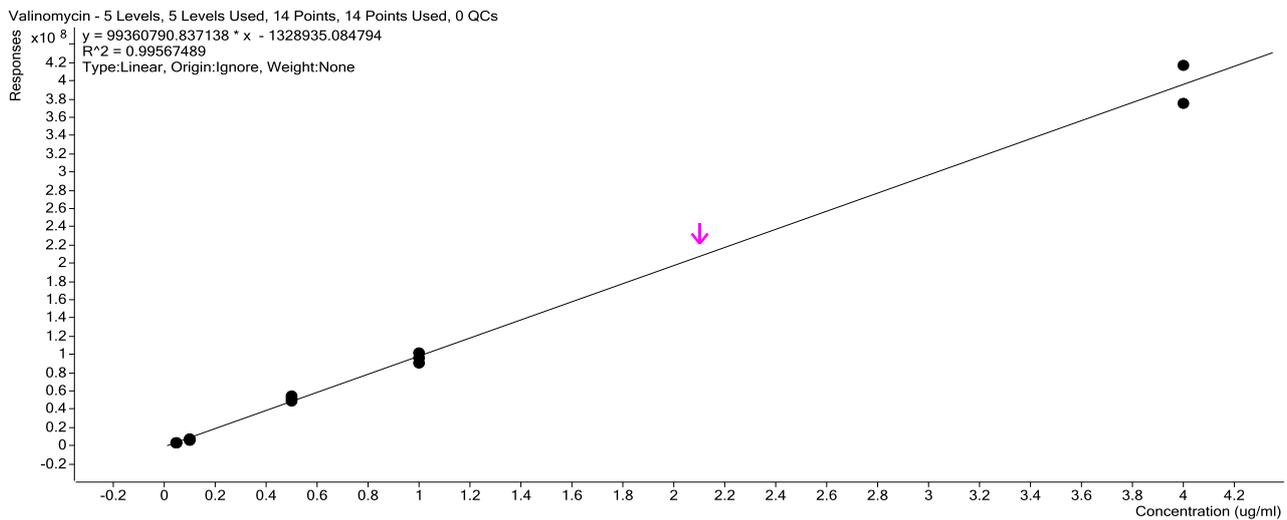
**Figure S3.** Calibration curve constructed to quantify valinomycin in *Streptomyces* sp. CBMAI 2042 extracts. The curve was evaluated in a range of 0.05-4.00  $\mu\text{g mL}^{-1}$  showing a linear regression coefficient of 0.99.
