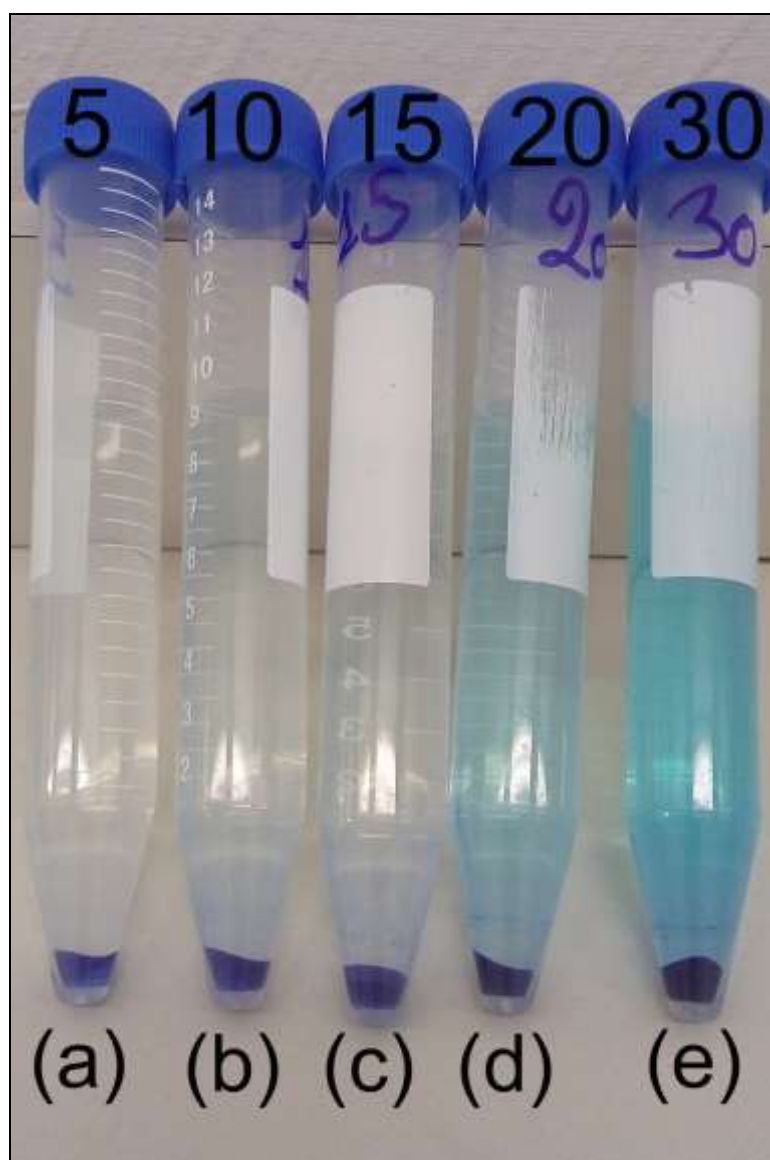
Figure S10. Image of samples of MB adsorption at equilibrium time 2 h, and 25 °C. Initial solutions (a) 5 mg L -1 ; (b) 10 mg L -1 ; (c) 15 mg L -1 ; (d) 20 mg L -1 ; (e) 30 mg L -1 .
