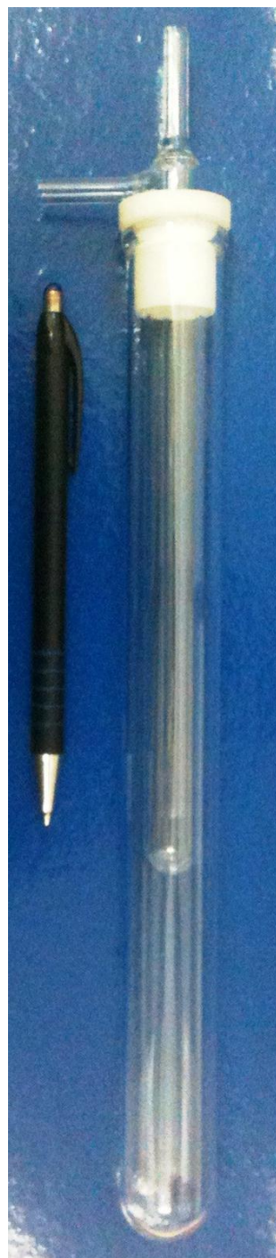
Figure S1. Schematic diagram of cold finger coupled to glass digester tube. 1: water inlet; 2: water outlet; 3: end cap of PTFE; 4: outlet to gas; 5: reaction flask.
