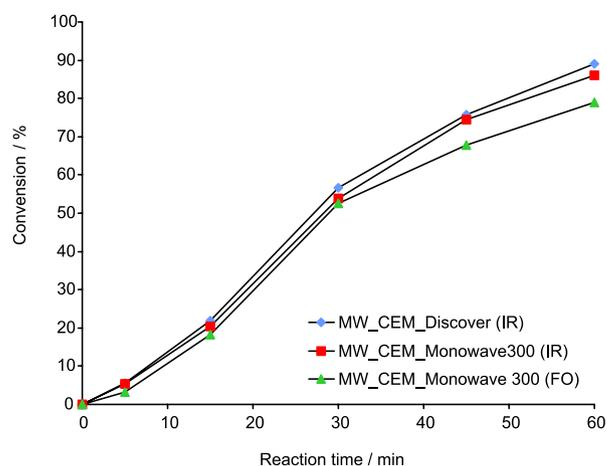
**Figure 4.** Conversion of oleic acid into ethyl oleate at different microwave equipments and temperature monitoring systems. Conversion based on GC-MS analysis.<sup>21</sup>
