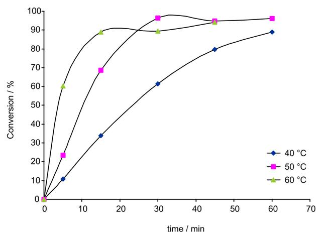
**Figure 1.** The influence of temperature on the conversion of oleic acid into ethyl oleate.
