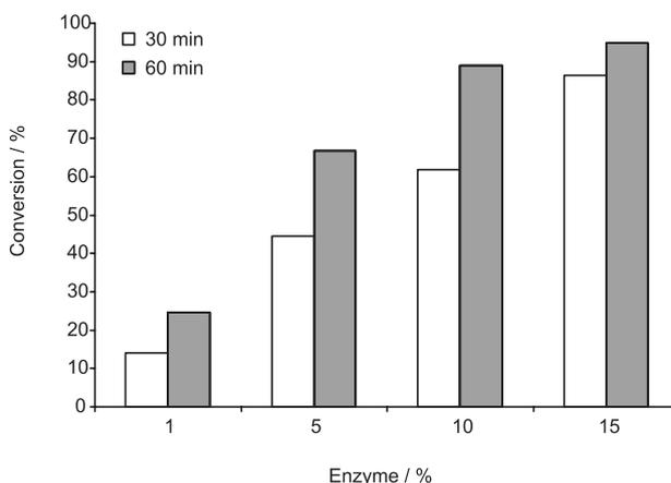
**Figure 3.** Effect of catalyst loading on the conversion of oleic acid into ethyl oleate.
