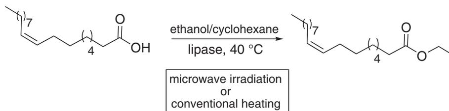
**Scheme 1.** Esterification reaction of oleic acid catalyzed by lipase.
