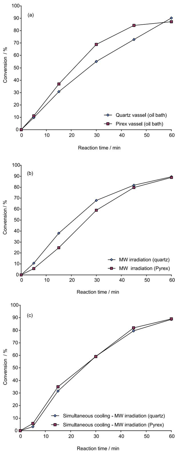
**Figure 2.** Results obtained in the esterification reaction under different heating protocols: (a) conventional heating and oil bath, (b) microwave irradiation and temperature control mode and (c) microwave irradiation and simultaneous cooling.
