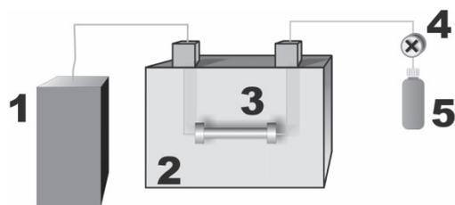
**Figure 2.** Schematic diagram of a Supercritical Fluid Extraction (SFE) apparatus. 1. Supercritical Fluid, 2. Oven, 3. Extraction Cell, 4. Restrictor. 5. Collector
