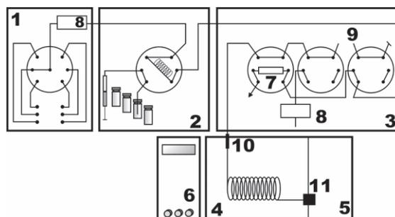
**Figure 11.** A fully automated analytical set up for the analysis of complex samples by on-line coupling Solid-Phase Extraction/Gas Chromatography with a Large Volume Injector and a Mass Spectrometer: SPE-LVI-GC-MS. 1. Solvent Delivery Unit, 2. Autosampler (MIDAS), 3. Automated SPE Unit (PROSPEKT) 4. GC, 5. MS, 6. Large Volume Injector (OPTIC), 7. SPE cartridge, 8. Pump, 9. Nitrogen gas, 10. PTV Injector, 11. Interface.
