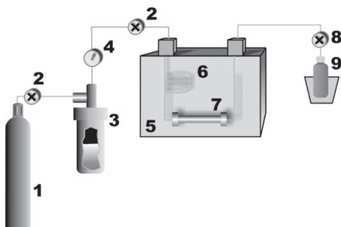
**Figure 3.** Schematic diagram of a Subcritical Water Extraction (SWE) apparatus. 1. N<sub>2</sub> Tank, 2. Valve, 3. Pressurized Solvent Vessel, 4. Pressure Monitor, 5. Oven, 6. Pre-heater, 7. Extraction Cell, 8. Restrictor, 9. Collector.
