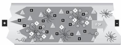
**Figure 8.** Schematic drawing of a MECC column emphasizing micelle formation inside the column. The micelles will show preference to retain some analytes while not retaining (or retaining less) the others, according to their relative affinities represented here by different shapes.
