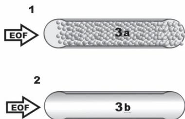
**Figure 9.** Capillary Electrochromatography (CEC) Columns. 1. Packed CEC column, 2. Open Tubular CEC column, 3a. Packing Material, 3b. Wall Coating.
