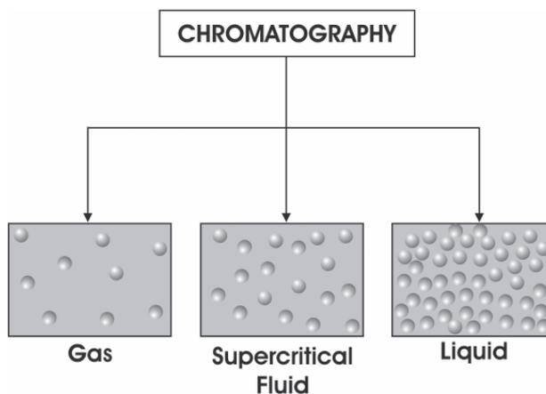
**Figure 4.** Classification of the chromatographic techniques according to the physical state of the mobile phase.
