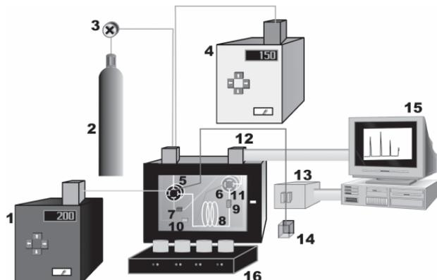
**Figure 12.** General view of a Unified Chromatographic Apparatus. 1. High Pressure Pump for Supercritical Fluid Delivery; 2. Gas Cylinder. 3. Pressure Control Valve; 4. HPLC Pump; 5. Selection Valve; 6. Restrictor Selection Valve; 7. Connector; 8. Column; 9. Restrictor; 10. Oven; 11. Retention Gap; 12. GC Detector; 13. LC Detector; 14. Sample Waste; 15. Data System; 16. Computerized Valve Controller System.
