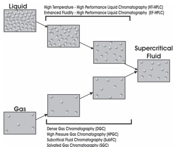
**Figure 10.** The role of the solvent in the separation sciences, with emphasis on various intermediate chromatographic techniques
