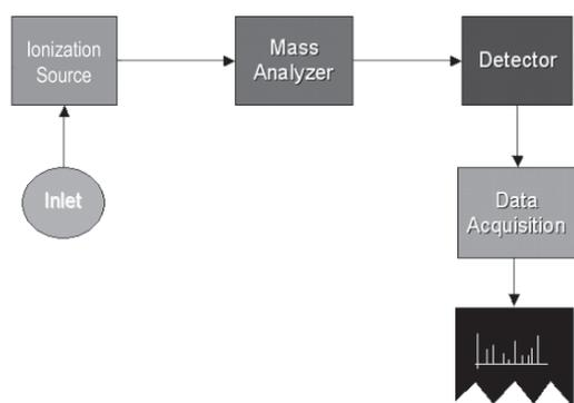
Figure 5. Schematic diagram of a Mass Spectrometer.
