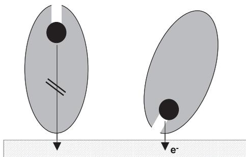
**Figure 3.** Effect of immobilized enzyme orientation on direct electron transfer.
