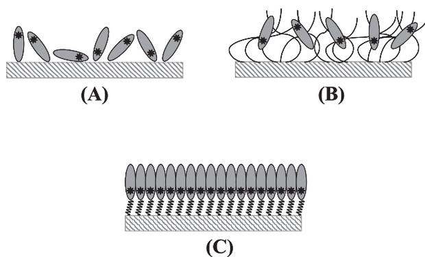
**Figure 4.** Representation of some methods used to achieve enzyme immobilization. (A) physical adsorption; (B) cross linking or inclusion in polyelectrolytes/conducting polymers; (C) oriented attachment to self-assembled monolayers.
