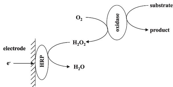
Figure 6. Schematics of coupling of two enzymes.
