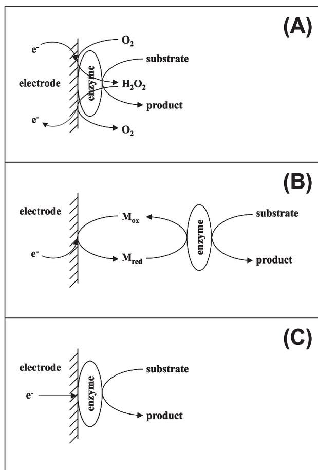
**Figure 2.** Schematic representation of different biosensor generations.
