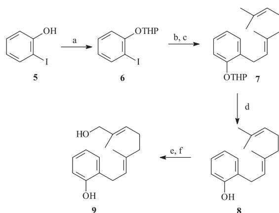
**Scheme 2.** (a) DHP (1.2 equiv.), PPTS (0.9 mmol%), CH<sub>2</sub>Cl<sub>2</sub>, Ar, 8 h, 95%. (b) *n*-BuLi, THF, TMEDA, -78 to -25 °C. (c) THF, -98 °C, geranyl bromide **4**, THF, -78 °C, two steps 95%. (d) MeOH, PPTS (0.9 mmol), 50 °C, 12h, 93%. (e) SeO<sub>2</sub>/SiO<sub>2</sub> (10% m/m), *t*-BuO<sub>2</sub>H (2 equiv.), CH<sub>2</sub>Cl<sub>2</sub>, 25 °C. (f) NaBH<sub>4</sub>, THF (1/20 v/v), -10 °C, two steps 47%.
