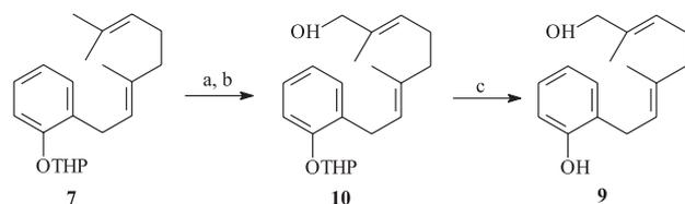
**Scheme 3.** (a) SeO<sub>2</sub>/SiO<sub>2</sub> (10% m/m), *t*-BuO<sub>2</sub>H (2 equiv.), CH<sub>2</sub>Cl<sub>2</sub>, 25 °C, 48 h. (b) NaBH<sub>4</sub>, MeOH/THF (1/20, v/v), -10 °C, 20 min, two steps 58%. (c) MeOH, PPTS (0.9 mmol), 50 °C, 12 h, 92%.
