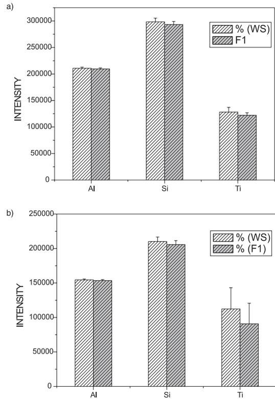
**Figure 6.** Emission intensities and relative standard deviations for Al, Si, and Ti (n = 3). Slurries prepared from IPT-42 using (a) Na<sub>2</sub>CO<sub>3</sub> or (b) LiBO<sub>2</sub>. WS – without separation of particle sizes and F1 – particles sizes lower than 37 μm.
