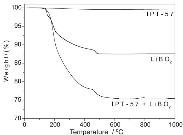
**Figure 3.** Thermogravimetric curves for LiBO<sub>2</sub> and for IPT-57 ground without modifier and with LiBO<sub>2</sub>.
