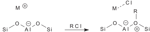
Scheme 2. Reaction of an alkylchloride with a metal-exchanged zeolite. Formation of alkoxides.
