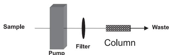
**Figure 1.** Field sampling system for determination of cadmium and nickel in fresh water samples.
