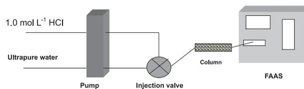
**Figure 2.** On-line elution system for determination of cadmium and nickel.
