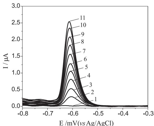
**Figure 2.** SWV responses for several concentrations of Fenitrothion in  $0.1 \text{ mol L}^{-1}$  BR buffer at pH 10.5: (1) supporting electrolyte, (2) 0.09, (3) 0.18, (4) 0.28, (5) 0.37, (6) 0.45, (7) 0.54, (8) 0.63, (9) 0.72, (10) 0.80, (11)  $0.89 \text{ mmol L}^{-1}$ ,  $f = 100 \text{ s}^{-1}$ ,  $a = 50 \text{ mV}$  and  $\Delta E_s = 2 \text{ mV}$ .
