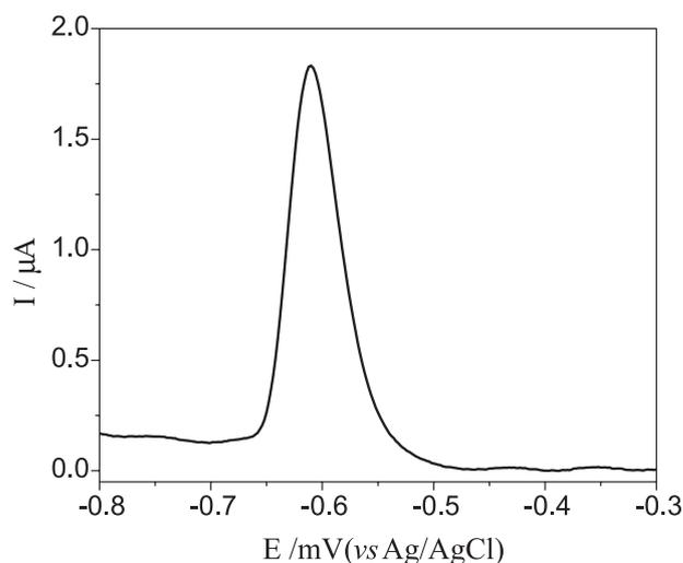
**Figure 1.** SWV responses for  $0.631 \mu\text{mol L}^{-1}$  Fenitrothion in 0.1 mol L<sup>-1</sup> BR buffer at pH 10.5,  $\Delta E_s = 2$  mV,  $a = 50$  mV,  $f = 100$  s<sup>-1</sup>.
