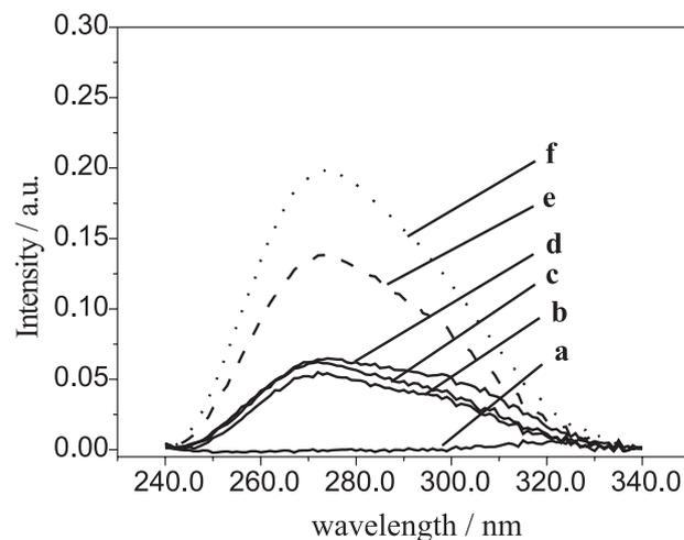
**Figure 5.** UV-Vis spectrum for the commercial formulation samples (diluted to labeled  $1.1 \text{ mmol L}^{-1}$  Fenitrothion). (a)  $0.1 \text{ mol L}^{-1}$  BR buffer (blank); (b) Sumithion 500CE; (c) Periphos CE; (d) Sumithion UBV; (e) after addition of  $1.01 \text{ mmol L}^{-1}$  Fenitrothion; (f) after addition of  $2.02 \text{ mmol L}^{-1}$  Fenitrothion.
