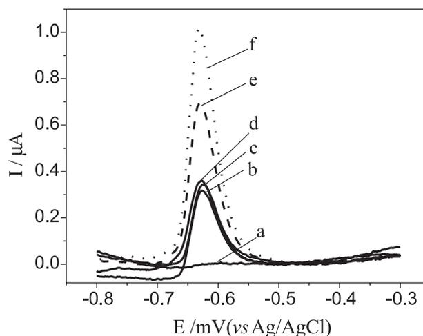
**Figure 3.** SWV responses for commercial formulation samples (diluted to labeled  $0.09 \text{ mmol L}^{-1}$  Fenitrothion). (a)  $0.1 \text{ mol L}^{-1}$  BR buffer (blank); (b) Sumithion 500CE; (c) Sumithion UBV; (d) Periphos CE; (e) after addition of  $0.09 \text{ mmol L}^{-1}$  Fenitrothion; (f) after addition of  $0.18 \text{ mmol L}^{-1}$  Fenitrothion.  $f = 100 \text{ s}^{-1}$ ,  $a = 50 \text{ mV}$  and  $\Delta E_s = 2 \text{ mV}$ .
