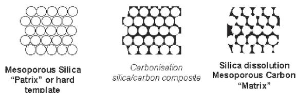
Figure 1. Preparation of mesoporous carbons by nano-casting.
