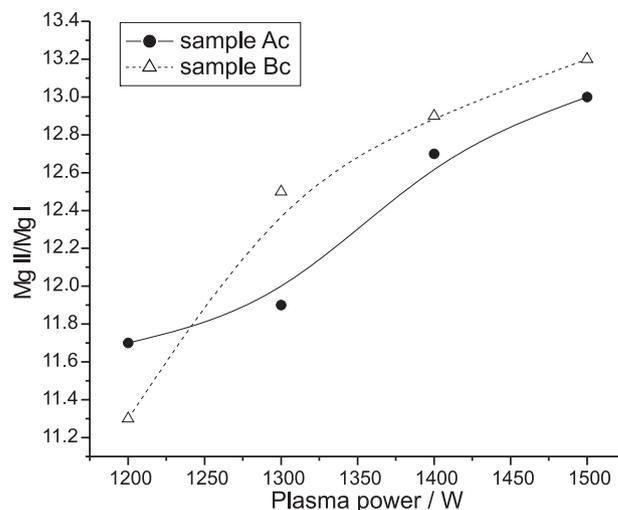
**Figure 2.** Mg II/Mg I ratio for samples "Ac" and "Bc". Operational conditions: nebulization flow rate: 0.5 L min<sup>-1</sup> and auxiliary gas flow rate: 0.5 L min<sup>-1</sup>.
