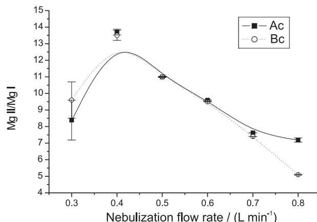
**Figure 1.** Mg II/Mg I ratio for samples "Ac" and "Bc". Operational conditions: plasma power: 1300 W and auxiliary gas flow rate: 0.5 L min<sup>-1</sup>.
