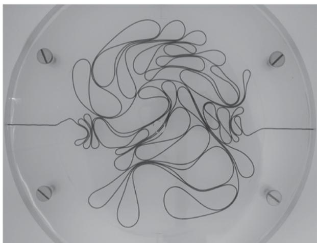
**Figure 1.** Example of heterogeneous hierarchical structures of loops obtained from the forced injection of a wire of copper with 1 mm diameter in a quasi-two-dimensional cavity of 100 mm of radius, and 1.1 mm of height.
