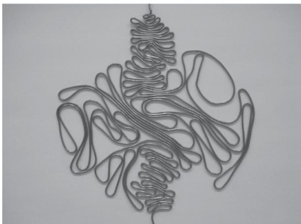
**Figure 2.** The same as in Figure 1, but for a wire of the alloy  $\text{Sn}_{0.60}\text{Pb}_{0.40}$  with 1.5 mm of diameter in a quasi-two-dimensional cavity of 75 mm of radius, and 1.6 mm of height.
