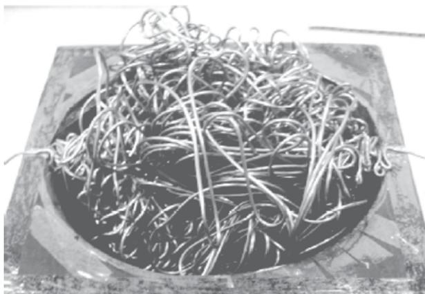
**Figure 3.** Example of a three-dimensional packing of wire obtained with the same method as in Figures 1 and 2, for the alloy wire of Figure 2, but in a spherical cavity of 75 mm of radius (the upper hemisphere of the cavity was removed to expose the structure).
