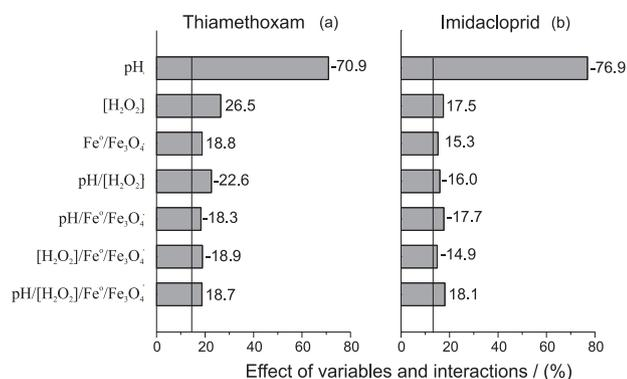
**Figure 2.** The Pareto chart for the degradation of: (a) Thiamethoxam; and (b) Imidacloprid. These plots were built based on the data displayed in Table 3.
