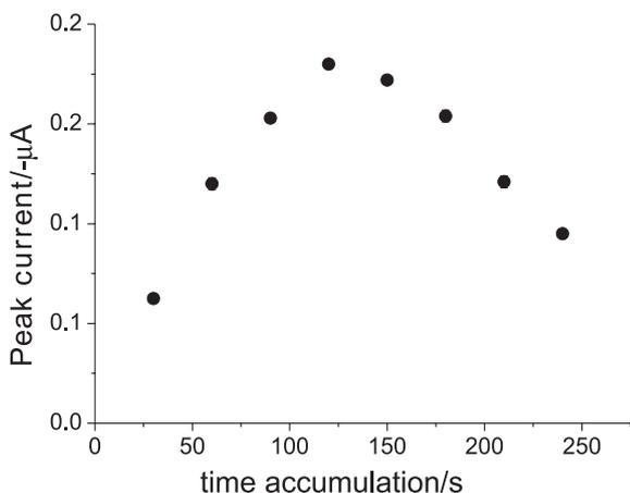
**Figure 3.** Influence of  $t_{\text{ads}}$  on the peak current of the Zn-Ox complex.  $C_{Zn(II)} = 10.0 \mu\text{g L}^{-1}$ ;  $\text{pH} = 7.3$ ;  $E_{\text{ads}} = 0.00 \text{ V}$ . 5 mV step amplitude, 25 mV pulse amplitude, and 25 Hz frequency.
