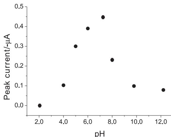
**Figure 1.** Influence of pH on the peak current of the Zn-Ox complex. Conditions:  $C_{\text{Zn(II)}} = 2.0$  µg L<sup>-1</sup>;  $C_{\text{ox}} = 10$  µmol L<sup>-1</sup>;  $t_{\text{ads}} = 60$  s;  $E_{\text{ads}} = 0.00$  V. 5 mV step amplitude, 25 mV pulse amplitude and 25 Hz frequency.
