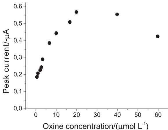
**Figure 2.** Influence of oxine concentration on the peak current of the Zn-Ox complex. Conditions:  $C_{Zn(II)} = 10.0 \mu\text{g L}^{-1}$ ;  $\text{pH} = 7.3$ ;  $t_{\text{ads}} = 60 \text{ s}$ ;  $E_{\text{ads}} = 0.00 \text{ V}$ . 5 mV step amplitude, 25 mV pulse amplitude and 25 Hz frequency.
