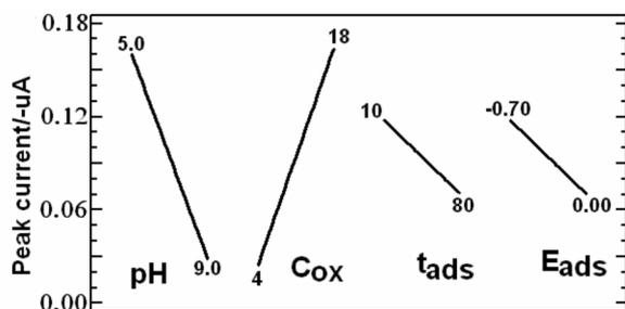
**Figure 4.** Influence of pH,  $C_{\text{ox}}$ ,  $t_{\text{ads}}$  and  $E_{\text{ads}}$  in the response in the  $2^4$  factorial design.  $C_{\text{Zn(II)}} = 10.0 \mu\text{g L}^{-1}$ .
