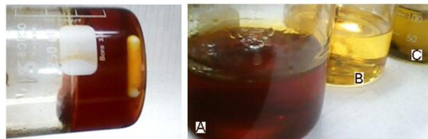
**Figure 12.** Accelerated aged FR3<sup>®</sup> oil samples A, B and C.
