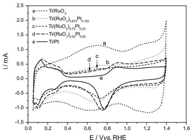
**Figure 1.** Cyclic voltammograms of  $\text{Ti}/(\text{RuO}_2)_{(x)}\text{Pt}_{(1-x)}$  electrodes in 0.1  $\text{mol L}^{-1}$   $\text{HClO}_4$ ,  $v = 50 \text{ mV s}^{-1}$ ,  $T = 25 \text{ }^\circ\text{C}$ .
