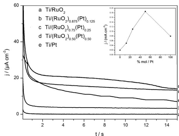
**Figure 4.** Chronoamperometric measurements for 0.5 mol L<sup>-1</sup> ethanol in 0.1 mol L<sup>-1</sup> HClO<sub>4</sub> on  $\text{Ti}/(\text{RuO}_2)_x\text{Pt}_{(1-x)}$  electrodes.  $E_{\text{ox}} = 0.5\text{ V}$ .  $T = 25\text{ }^\circ\text{C}$ . Inset: optimal ratio of Pt load.
