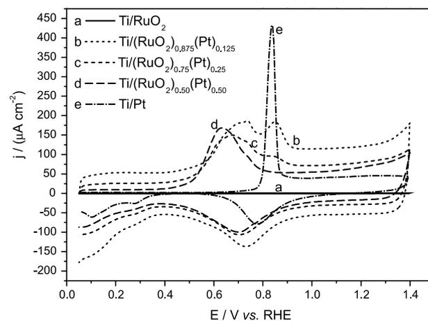
**Figure 2.** Cyclic voltammograms obtained for the oxidative stripping of a CO monolayer on  $\text{Ti}/(\text{RuO}_2)_{(x)}\text{Pt}_{(1-x)}$  electrodes in 0.1  $\text{mol L}^{-1}$   $\text{HClO}_4$ ,  $v = 50 \text{ mV s}^{-1}$ ,  $T = 25 \text{ }^\circ\text{C}$ .
