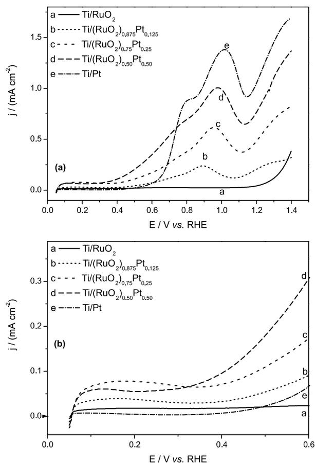
**Figure 3.** Cyclic voltammograms obtained for (a) electrooxidation of 0.5 mol L<sup>-1</sup> ethanol in 0.1 mol L<sup>-1</sup> HClO<sub>4</sub> and (b) presenting the shifting of the onset potential during ethanol electrooxidation on Ti/(RuO<sub>2</sub>)<sub>(x)</sub>Pt<sub>(1-x)</sub> electrodes. v = 50 mV s<sup>-1</sup>, T = 25 °C.
