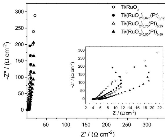
**Figure 6.** Nyquist plots of EIS for 0.5 mol L<sup>-1</sup> ethanol in 0.1 mol L<sup>-1</sup>  $\text{HClO}_4$  reaction on  $\text{Ti}/(\text{RuO}_2)_x\text{Pt}_{(1-x)}$  electrodes electrochemically polarized at 0.9 V.  $T = 25^\circ\text{C}$ .
