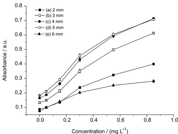
**Figure 3.** Effect of the optical pathlength: (a), (b), (c), (d) and (e) correspond to the flow cell length of 2, 3, 4, 5 and 6 mm, respectively. Results are average of three consecutive measurements.
