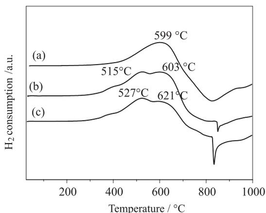
**Figure 6.** Curves of temperature programmed reduction for the (a) 5IAC, (b) 10IAC and (c) 15IAC samples (activated carbon-supported magnetite). The numbers represent the iron amount (wt.%) in the solids.
