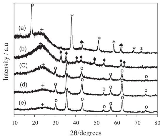
**Figure 2.** X-ray diffractograms for the (a) AC sample (activated carbon), and for the (b) 2.5IAC, (c) 5IAC (d) 10IAC and (e) 15IAC samples (activated carbon-supported iron oxide). The numbers represent the iron amount (wt.%) in the solids. (♣): magnesium oxide (MgO); (\*) magnesium carbide ( $\text{Mg}_2\text{C}_3$ ); (+) activated carbon; (O) magnetite ( $\text{Fe}_3\text{O}_4$ ); (◆) hematite ( $\text{Fe}_2\text{O}_3$ ).
