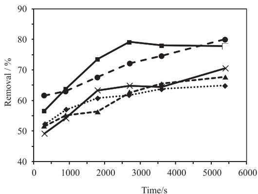
**Figure 8.** Methylene blue removal by adsorption on the catalysts as a function of time during the Fenton reaction, AC sample (x) (activated carbon), and 2.5IAC (◆), 5IAC (▲), 10IAC (●) and 15IAC (■) samples (activated carbon-supported iron oxide). The numbers represent the iron amount (wt.%) in the solids.
