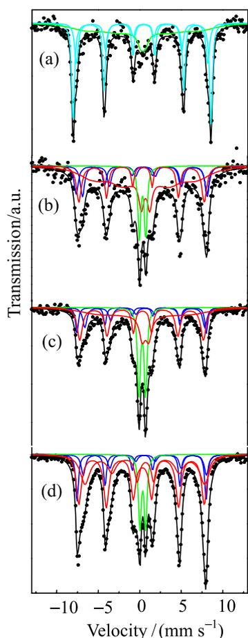
**Figure 3.** Mössbauer spectra for the (a) 2.5 IAC, (b) 5IAC, (c) 10IAC and (d) 15IAC samples (activated carbon-supported iron oxide). The numbers represent the iron amount (wt.%) in the solids. The blue lines represent magnetically blocked magnetite or hematite, the red one the relaxing magnetite or hematite and the green ones represent supermagnetic hematite.
