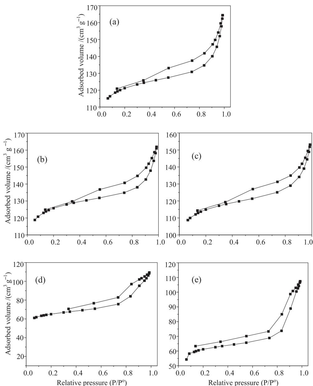
**Figure 5.** Adsorption and desorption isotherms for the (a) AC sample (activated carbon), and for the (b) 2.5IAC, (c) 5IAC, (d) 10IAC and (e) 15IAC sample (activated carbon-supported iron oxide). The numbers represent the iron amount (wt.%) in the solids.
