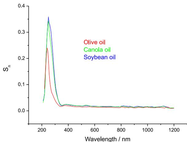
**Figure 3.** Photoacoustic  $S_n$  spectra of olive, canola and soybean oils.
