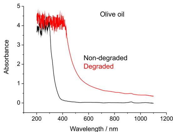
**Figure 7.** Conventional absorbance spectra of non-degraded and degraded olive oil.
