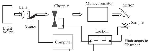
**Figure 2.** Experimental setup of the photothermal spectrometer.
