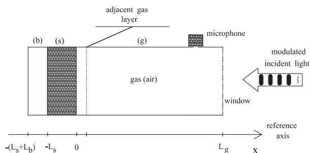
**Figure 1.** Sketch of the closed cylindrical photoacoustic chamber showing the adjacent gas layer which acts as an acoustic piston. The letters: b = backing, s = sample, g = gas,  $L_s$  = sample thickness,  $L_g$  = gas layer thickness,  $L_b$  = backing layer thickness and X = reference axis.
