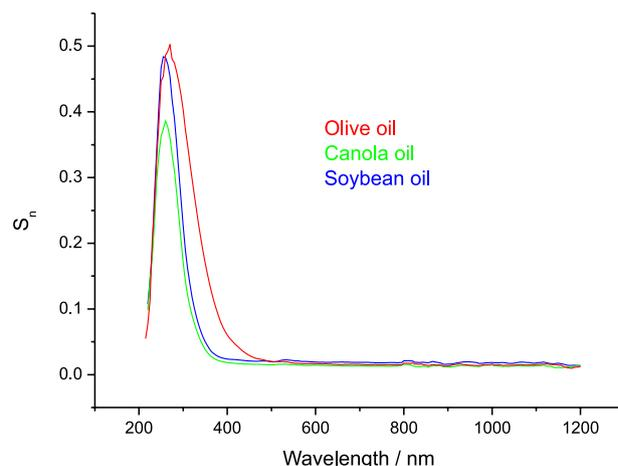
**Figure 5.** Photoacoustic  $S_n$  spectra of degraded olive, canola and soybean oils.
