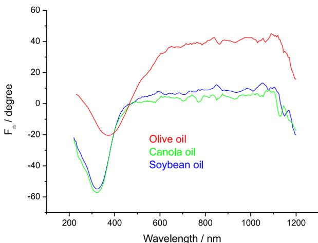
**Figure 6.** Photoacoustic  $F_n$  spectra of degraded olive, canola and soybean oils.
