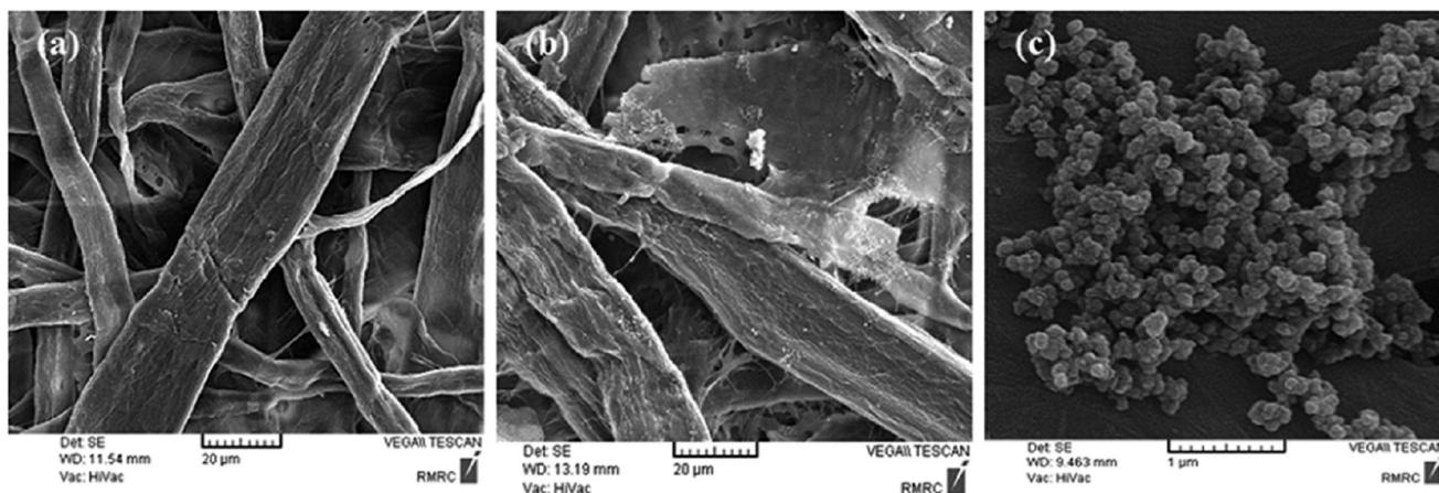
**Figure 1.** SEM images of the filter paper before polymerization (a) and PANI/PPY-cellulose nanocomposite with low (b) and high (c) magnifications.
