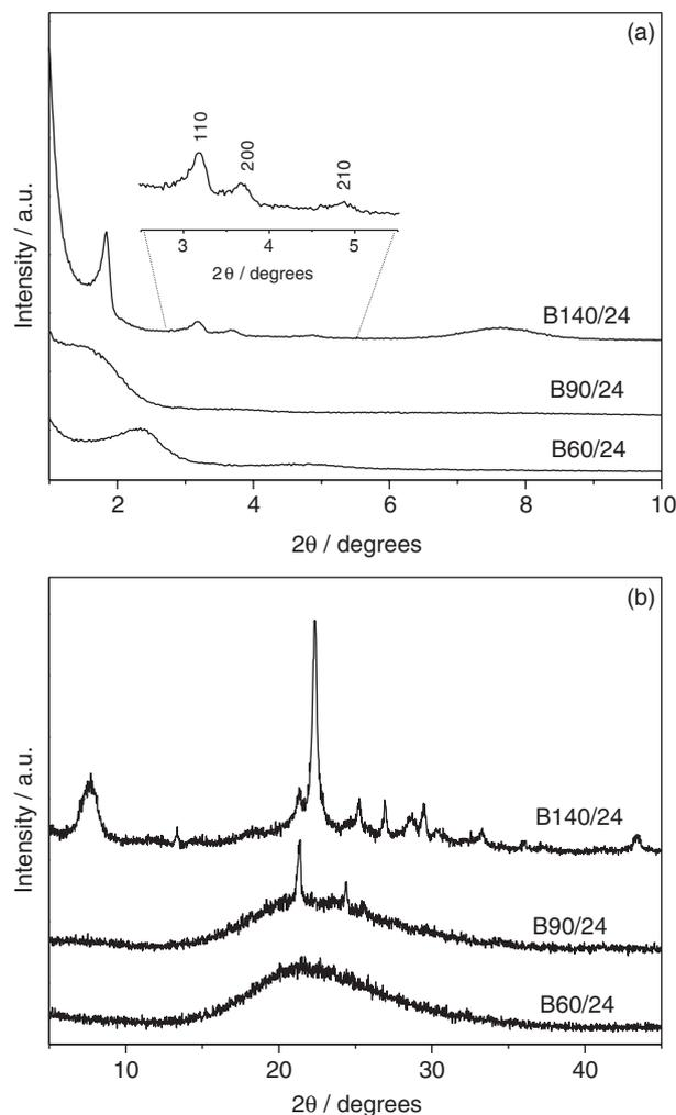
**Figure 1.** X-ray diffractograms of samples obtained by aging the seed gel of beta zeolite at different temperatures (60, 90 and 140 °C) for 24 h, in the region of (a) small and (b) high angles.
