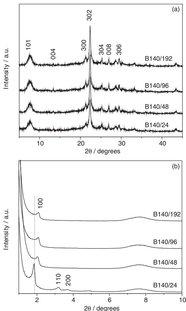
**Figure 3.** X-ray diffractograms for calcined samples obtained at different times (24, 48, 96 and 192 h) of seed gel aging at 140 °C, in the region of (a) high angles and (b) small angles.
