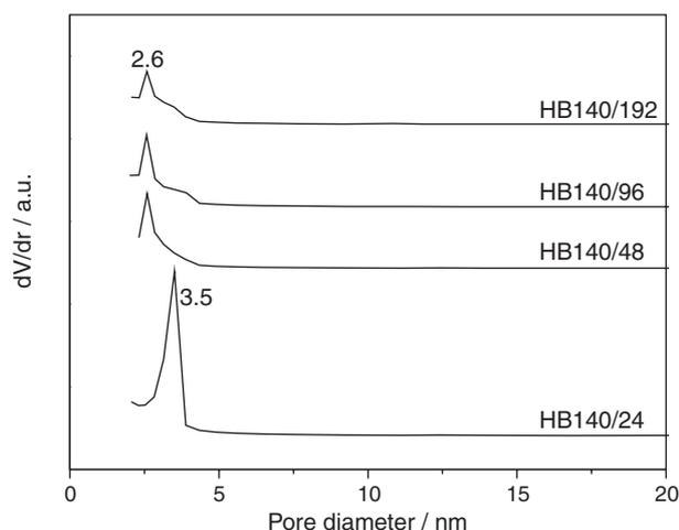
**Figure 6.** Pore size distribution for the acidic form (H) of beta zeolite/MCM-41 materials obtained at different aging times (24, 48, 96 and 192 h) of the seed gel at 140 °C.
