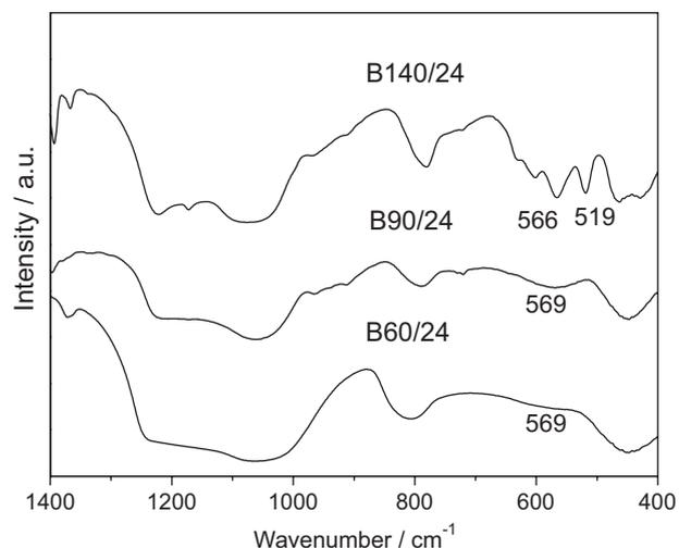
**Figure 2.** FTIR spectra of samples obtained by aging the seed gel of beta zeolite at different temperatures (60, 90 and 140 °C) for 24 h; enlargement from 400 to 1400 cm<sup>-1</sup>.
