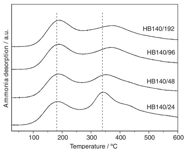
**Figure 7.** Number of moles of ammonia desorbed *per* gram of solid as a function of temperature, for beta zeolite/MCM-41 materials obtained at different aging times (24, 48, 96 and 192 h) of the seed gel at 140 °C.
