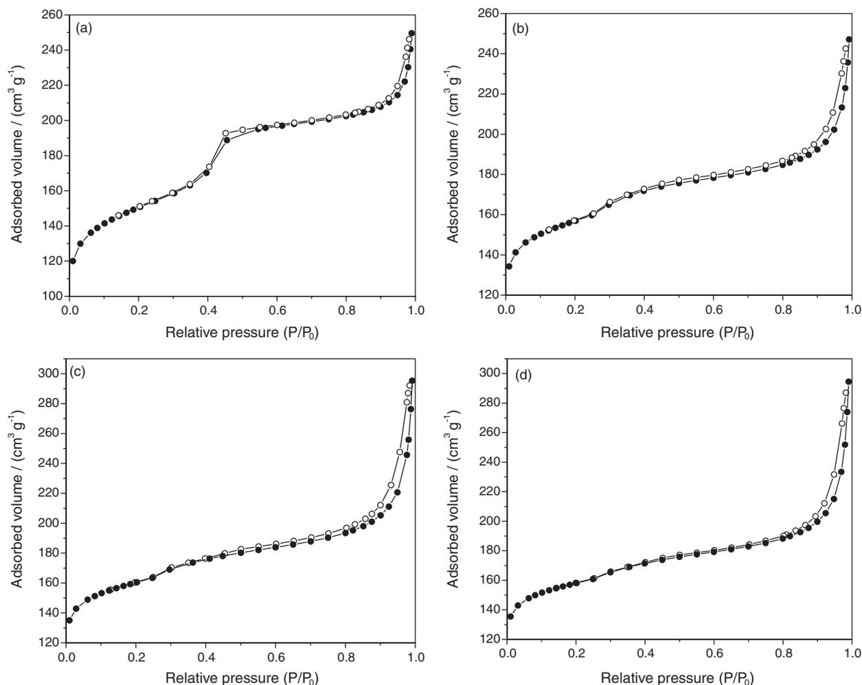
**Figure 5.** Nitrogen adsorption (●) and desorption (○) isotherms for the acidic form (H) of the mesostructured beta zeolite obtained at different aging times (24, 48, 96 and 192 h) of the seed gel at 140 °C. (a) HB140/24; (b) HB140/48; (c) HB140/96 and (d) HB140/192.
