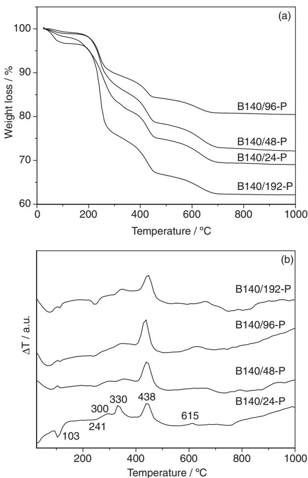
**Figure 4.** Curves of (a) thermogravimetry and (b) differential thermal analysis for the as-synthesized beta zeolite/MCM-41 materials (P) obtained at different aging times (24, 48, 96 and 192 h) of the seed gel at 140 °C.
