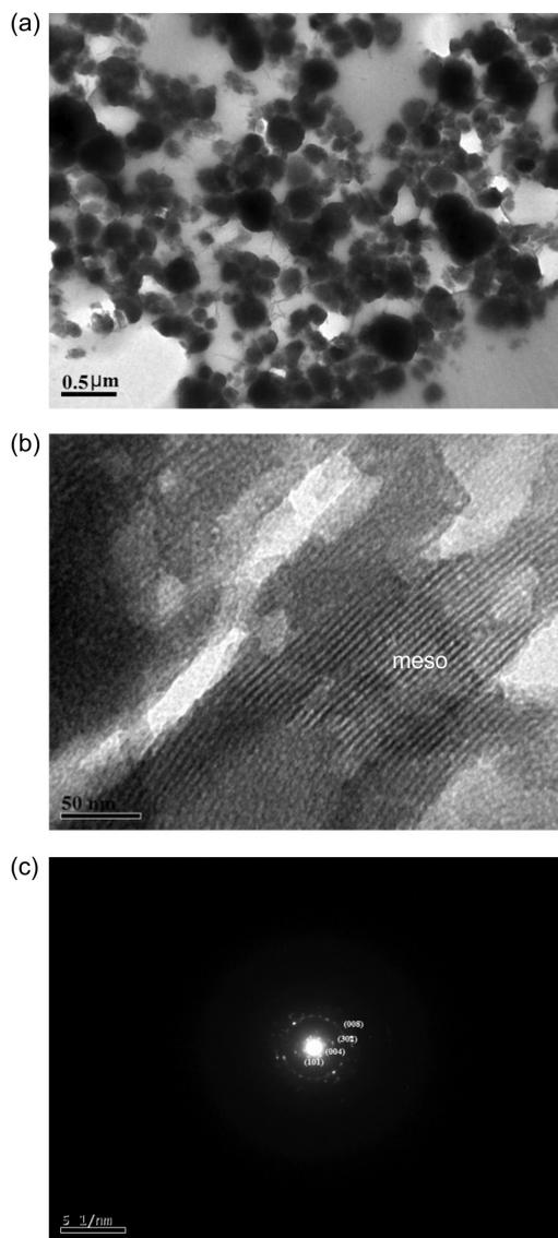
**Figure 8.** (a) TEM image of HB140/192 sample; (b) TEM image of HB140/96 sample showing the mesophase domain and (c) electron diffractogram showing the domain corresponding to the crystalline phase.
