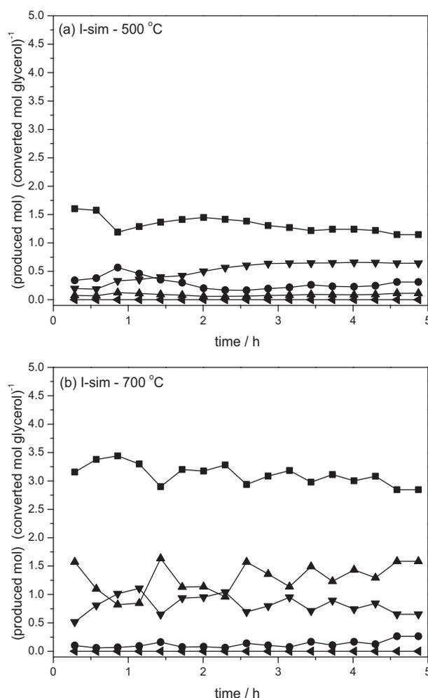
**Figure 8.** Gaseous products formed during the steam reforming of glycerol, on 10Ni30LaSi (I-sim): (a) 500 °C and (b) 700 °C. (■) H<sub>2</sub>; (●) CH<sub>4</sub>; (▲) CO; (▼) CO<sub>2</sub>; (◄) C<sub>2</sub>H<sub>4</sub>).
