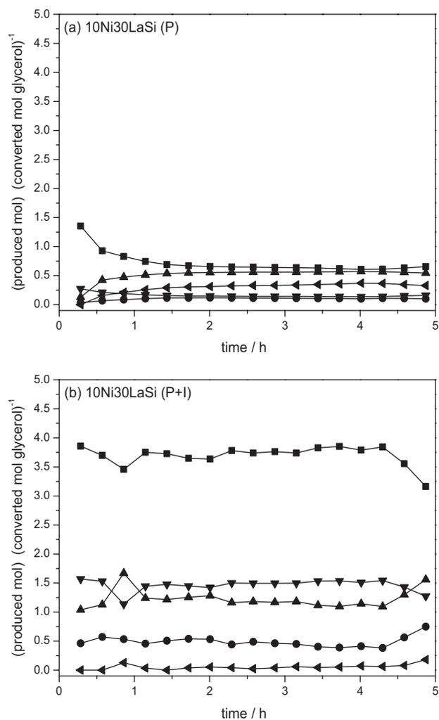
**Figure 4.** Gaseous products formed during the steam reforming of glycerol: (a) P, (b) P + I. (■) H<sub>2</sub>; (●) CH<sub>4</sub>; (▲) CO; (▼) CO<sub>2</sub>; (◄) C<sub>2</sub>H<sub>4</sub>.
