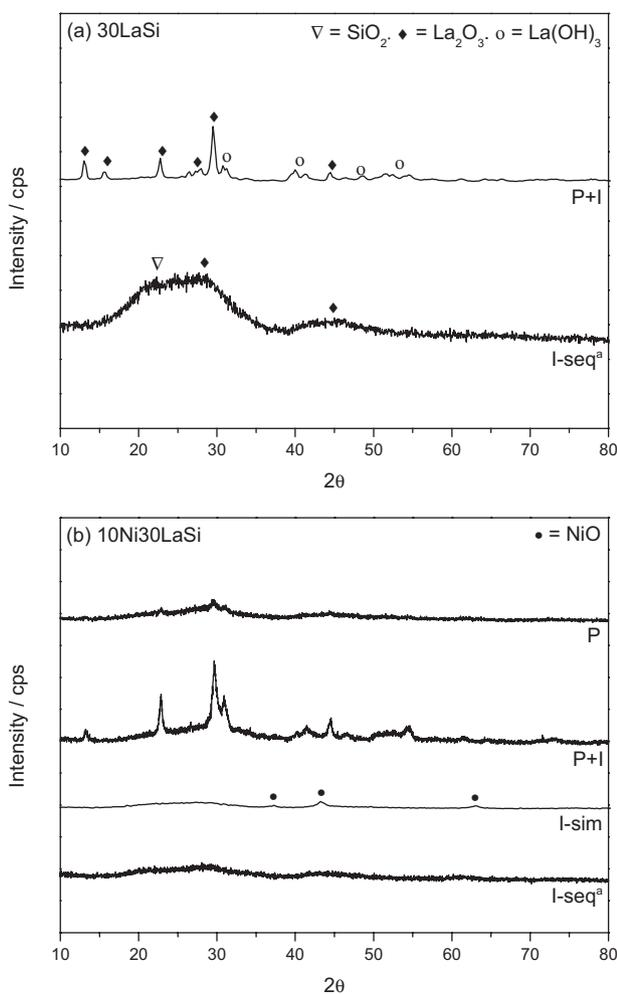
**Figure 1.** XRD patterns of (a) supports and (b) catalysts. <sup>a</sup>Data based on Thyssen *et al.*<sup>10</sup>
