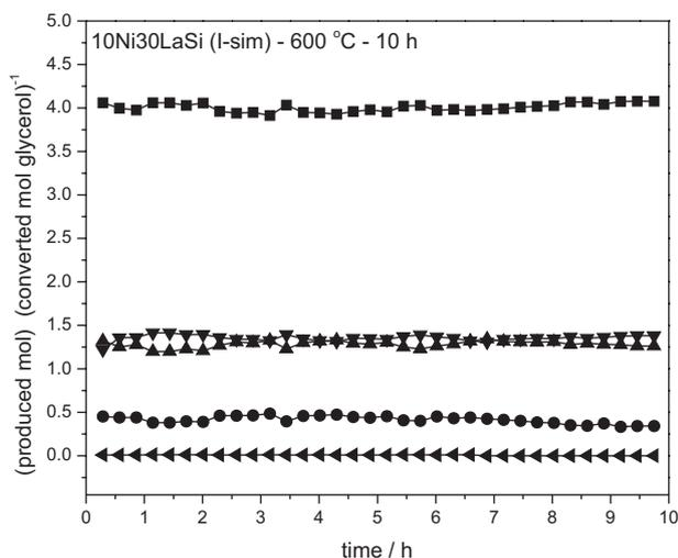
**Figure 9.** Gaseous products formed during the reaction of steam reforming of glycerol on 10Ni30LaSi (I-sim) over 10 h at 600 °C. (■ H<sub>2</sub>; ● CH<sub>4</sub>; ▲ CO; ▼ CO<sub>2</sub>; ◀ C<sub>2</sub>H<sub>4</sub>).
