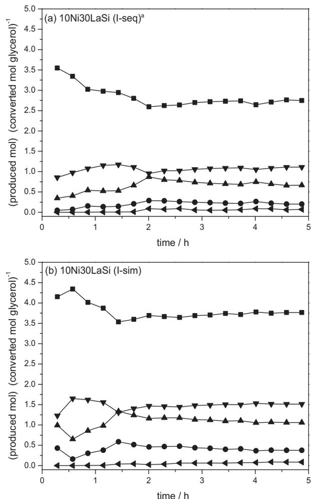
**Figure 5.** Gaseous products formed during the steam reforming of glycerol: (a) I-seq<sup>a</sup> and (b) I-sim. (■) H<sub>2</sub>; (●) CH<sub>4</sub>; (▲) CO; (▼) CO<sub>2</sub>; (◄) C<sub>2</sub>H<sub>4</sub>. <sup>a</sup>Data based on Thyssen *et al.*<sup>10</sup>
