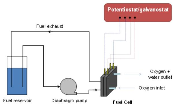
Figure 1. Experimental setup used in this study.
