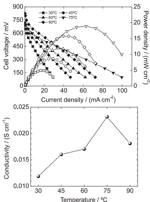
**Figure 2.** (a) fuel cell performance for different temperatures in the alkaline DGFC (glycerol concentration: 1 mol L<sup>-1</sup>; KOH concentration: 4 mol L<sup>-1</sup>; oxygen as comburent with a flow rate of 20 mL min<sup>-1</sup>; anode flow rate of 1 mL min<sup>-1</sup>) and (b) membrane conductivity at different temperatures.
