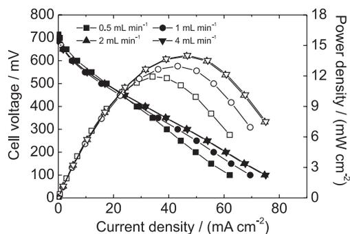
**Figure 6.** Fuel cell performance for different anode feed flow rates in the alkaline DGFC (glycerol concentration: 1 mol L<sup>-1</sup>; temperature: 60 °C; KOH concentration: 4 mol L<sup>-1</sup>; oxygen as comburent with a flow rate of 20 mL min<sup>-1</sup>).
