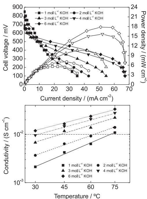
**Figure 5.** (a) fuel cell performance of the alkaline DGFC at different concentrations of KOH (glycerol concentration:  $1 \text{ mol L}^{-1}$ ; temperature:  $60 \text{ }^\circ\text{C}$ ; oxygen as comburent with a flow rate of  $20 \text{ mL min}^{-1}$ ; anode flow rate of  $1 \text{ mL min}^{-1}$ ); and (b) membrane conductivity at different KOH concentrations and cell temperatures.
