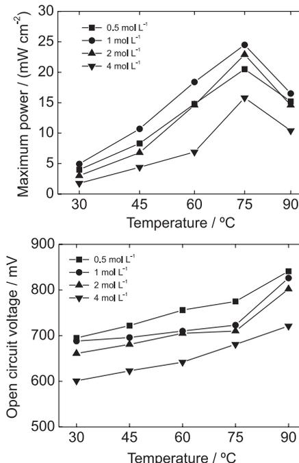
**Figure 4.** (a) maximum power density, and (b) open circuit voltage obtained in the alkaline DGFC at different temperatures and glycerol concentrations (KOH concentration: 4 mol L<sup>-1</sup>; oxygen as comburent with a flow rate of 20 mL min<sup>-1</sup>; anode flow rate of 1 mL min<sup>-1</sup>).
