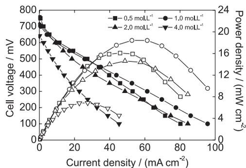
**Figure 3.** Fuel cell performance for different glycerol concentrations in the alkaline DGFC (temperature: 60 °C; KOH concentration: 4 mol L<sup>-1</sup>; oxygen as comburent with a flow rate of 20 mL min<sup>-1</sup>; anode flow rate of 1 mL min<sup>-1</sup>).
