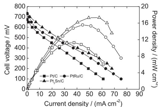
**Figure 7.** Fuel cell performance with different binary catalysts in the alkaline DGFC (glycerol concentration: 1 mol L<sup>-1</sup>; temperature: 60 °C; KOH concentration: 4 mol L<sup>-1</sup>; anode flow rate of 2 mL min<sup>-1</sup>; oxygen as comburent with a flow rate of 20 mL min<sup>-1</sup>).
