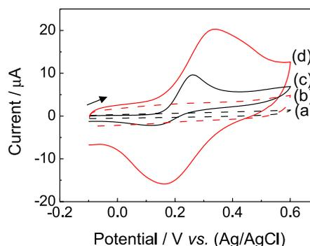
**Figure 3.** Cyclic voltammograms for a CPE (a, c) and a PVP-CPE sensor (b, d) in the absence (a, b) and presence (c, d) of  $1.0 \text{ mmol L}^{-1}$  quercetin in  $0.1 \text{ mol L}^{-1}$  phosphate buffer (pH 6.0),  $\nu = 100 \text{ mV s}^{-1}$ .
