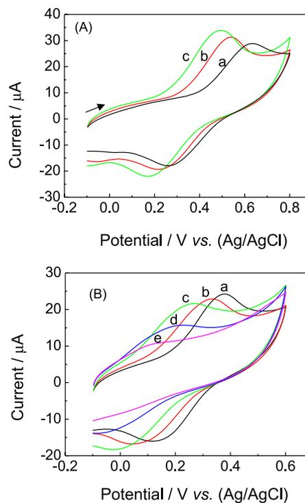
**Figure 5.** Cyclic voltammograms for  $1.0 \text{ mmol L}^{-1}$  quercetin in  $0.1 \text{ mol L}^{-1}$  Britton-Robinson buffer at the PVP-CPE sensor. (A) (a) pH 2.0, (b) pH 3.0 and (c) pH 4.0 and (B) (a) pH 5.0, (b) pH 6.0, (c) pH 7.0, (d) pH 8.0 and (e) pH 9.0;  $\nu = 100 \text{ mV s}^{-1}$ .
