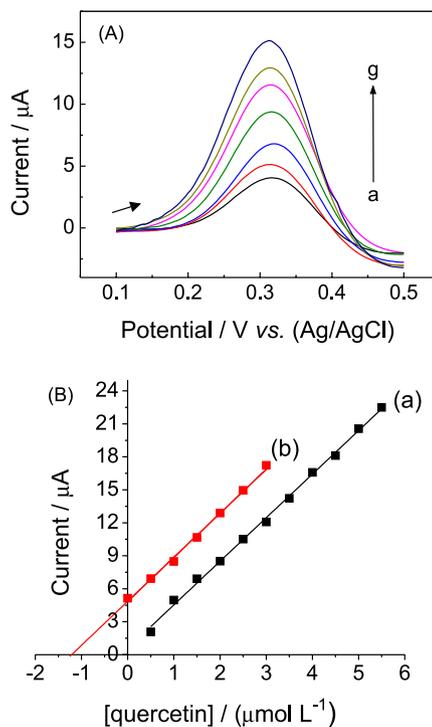
**Figure 10.** (A) Square-wave voltammograms for (a) sample alone, (b-g) sample with successive additions of 0.5 μmol L<sup>-1</sup> quercetin standard solution in 0.1 mol L<sup>-1</sup> acetate buffer (pH 5.0) obtained at the PVP-CPE sensor,  $f = 60$  Hz,  $a = 100$  mV and  $\Delta E_s = 4$  mV; (B) (a) the calibration curve and (b) the standard addition curve.
