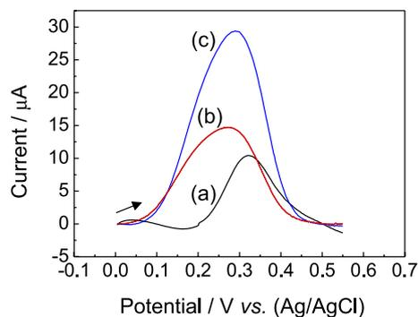
**Figure 8.** Voltammograms for 1.0  $\text{mmol L}^{-1}$  quercetin in 0.1  $\text{mol L}^{-1}$  acetate buffer (pH 5.0) at a PVP-CPE sensor obtained by: (a) LSV, (b) DPV and (c) SWV,  $v = 100 \text{ mV s}^{-1}$ .
