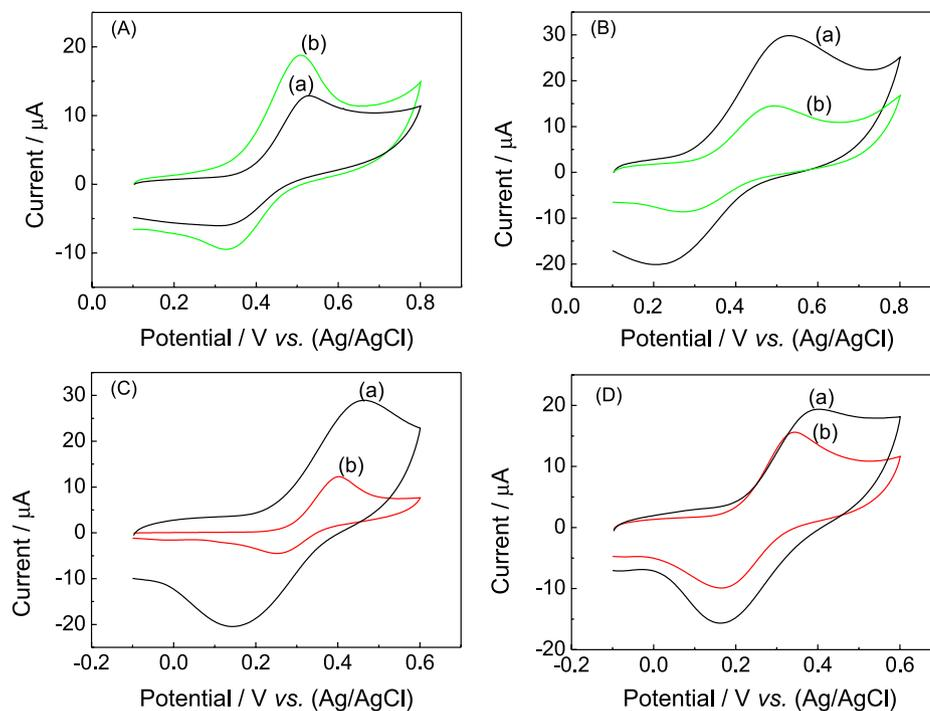
**Figure 6.** Cyclic voltammograms obtained at (A) pH 2.0 and (B) pH 3.0 in 0.1 mol L<sup>-1</sup> (a) Britton-Robinson and (b) phosphate buffers and (C) pH 4.0 and (D) pH 5.0 in 0.1 mol L<sup>-1</sup> (a) Britton-Robinson and (b) acetate buffers for 1.0 mmol L<sup>-1</sup> quercetin at the PVP-CPE sensor,  $\nu = 100$  mV s<sup>-1</sup>.
