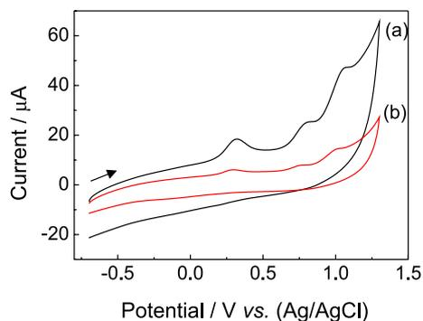
**Figure 2.** Cyclic voltammograms for  $1.0 \text{ mmol L}^{-1}$  quercetin in  $0.1 \text{ mol L}^{-1}$  phosphate buffer (pH 6.0) at a PVP-CPE sensor, (a) first cycle and (b) second cycle,  $\nu = 100 \text{ mV s}^{-1}$ .
