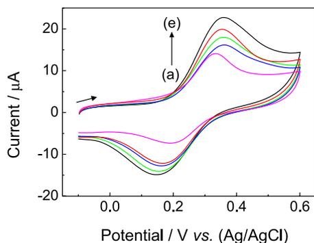
**Figure 4.** Cyclic voltammograms for  $1.0 \text{ mmol L}^{-1}$  quercetin in  $0.1 \text{ mol L}^{-1}$  phosphate buffer (pH 6.0) at the PVP-CPE sensors; (a-e) = 40, 30, 20, 10, 5% of PVP, respectively;  $\nu = 100 \text{ mV s}^{-1}$ .
