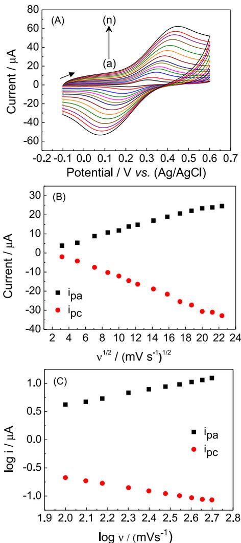
**Figure 7.** (A) Cyclic voltammograms for 1.0  $\text{mmol L}^{-1}$  quercetin in 0.1  $\text{mol L}^{-1}$  acetate buffer (pH 5.0) at the PVP-CPE sensor,  $v$  (a-j) = 10, 25, 50, 75, 100, 125, 150, 200, 250, 300, 350, 400, 450 and 500  $\text{mV s}^{-1}$ , respectively; (B) plot current vs.  $v^{1/2}$  and (C) plot  $\log i$  vs.  $\log v$ .
