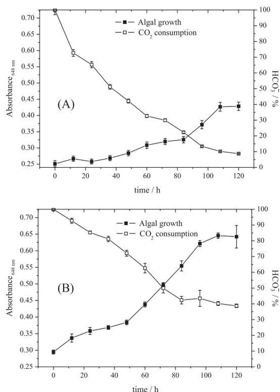
**Figure 2.** Effect of the gas supplementation on algal growth and carbon dioxide consumption observed for *C. vulgaris* cathodes. (A): Air 380 ppm; (B): pure CO<sub>2</sub>.
