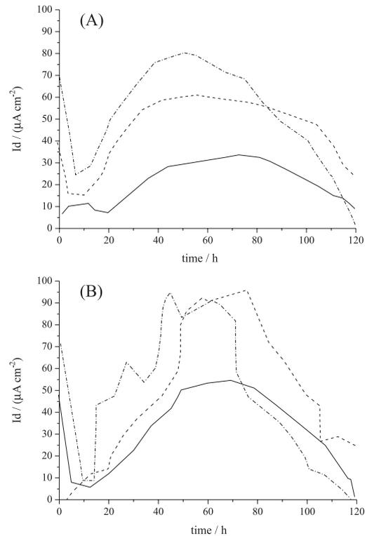
**Figure 6.** Effect of electron shuttles on the chronoamperometric profiles for HPSFC. No mediator (line); MB (dash); and BCG (dash-dot).
