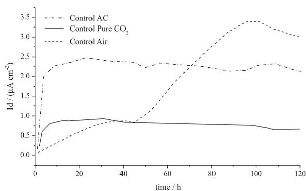
**Figure 4.** Chronoamperometric profiles obtained for control experiments using algae cathodes without aeration (AC) and with air or CO<sub>2</sub> supplementations.
