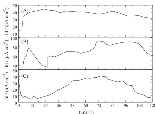
**Figure 3.** Chronoamperometric profiles observed for the algal cathode, supplemented with air (A) or pure CO<sub>2</sub> (B) and for bacterial anode (C).
