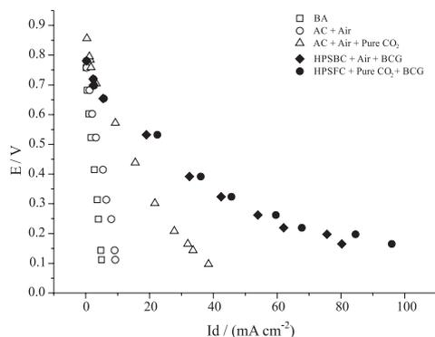
**Figure 7.** Polarization curves obtained for the evaluated systems at 60 h where the maxima current peaks were observed.
