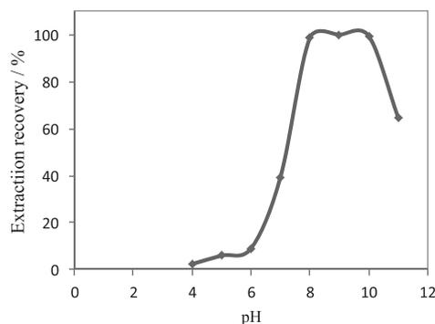
**Figure 1.** The effect of pH on extraction recovery of lead. (Sample volume: 25 mL; Triton X-114: 0.04 % (w/v); octanol: 10 µL; Pb: 100 µg L<sup>-1</sup>).
