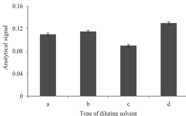
**Figure 3.** The effect of diluting solvent type on analytical signal of lead, (a) 1.0 mol L<sup>-1</sup> HNO<sub>3</sub> in THF; (b) 1.0 mol L<sup>-1</sup> HNO<sub>3</sub> in acetone; (c) 1.0 mol L<sup>-1</sup> HNO<sub>3</sub> in ethanol; (d) 1.0 mol L<sup>-1</sup> HNO<sub>3</sub> in methanol; sample volume: 25 mL; pH = 8.5; Triton X-114: 0.04% (w/v); octanol: 10  $\mu\text{L}$ ; Pb: 100  $\mu\text{g L}^{-1}$ .
