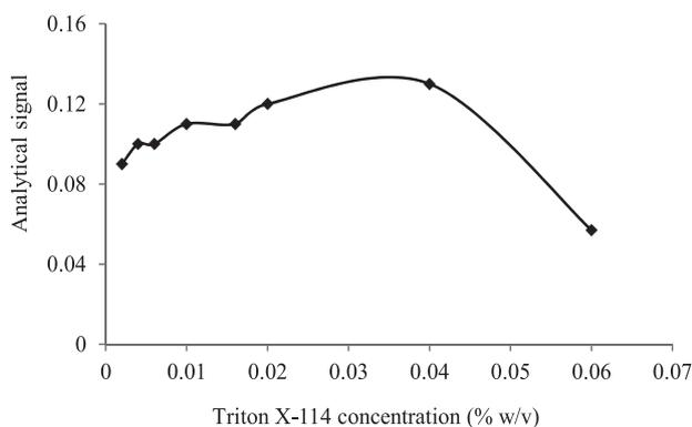
**Figure 2.** The effect of Triton X-114 concentration on analytical signal of lead. Sample volume: 25 mL; pH = 8.5; octanol: 10  $\mu\text{L}$ ; Pb: 100  $\mu\text{g L}^{-1}$ .
