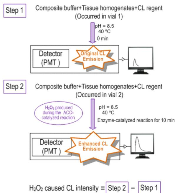
**Figure 2.** Analytical procedure for the acyl-CoA oxidase activity assay.
