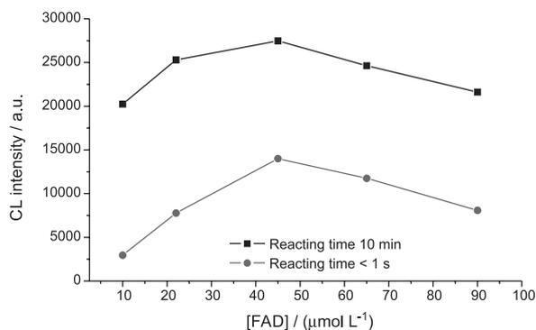
**Figure 4.** Effect of flavin adenine dinucleotide (FAD) concentration on chemiluminescence (CL) intensity.
