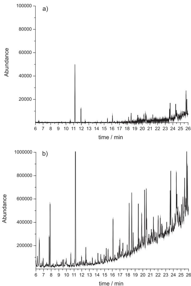
**Figure 3.** Chromatogram obtained by GC-MS-SCAN of the extracts free of chlorobenzenes: a) by SLE-PLT and b) by sohxlet extraction.
