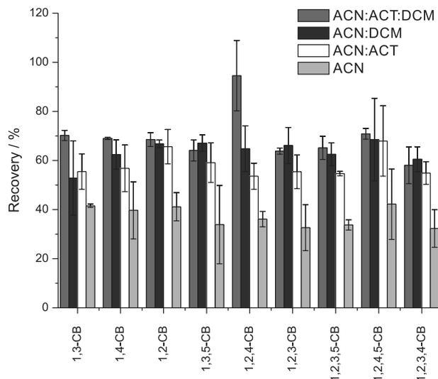
**Figure 1.** Influence of the extraction phase on the recovery percentage of chlorobenzenes (CB) in sewage sludge. ACN: acetonitrile; DCM: dichloromethane; ACT: ethyl acetate.
