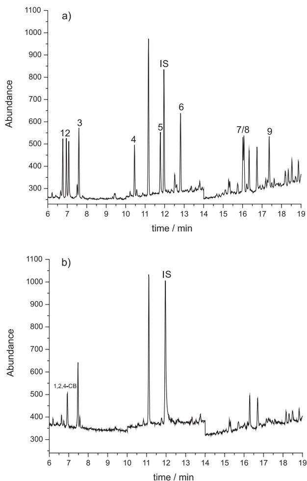
**Figure 2.** Chromatograms of the extract obtained after SLE-PLT: a) sludge extract spiked with chlorobenzenes from 6.6 to 20 µg L<sup>-1</sup>, b) sludge extract (blank). Identification of the peaks: (1) 1,3-CB, (2) 1,4-CB, (3) 1,2-CB, (4) 1,3,5-CB, (5) 1,2,4-CB, IS, (6) 1,2,3-CB, (7) 1,2,3,5-CB, (8) 1,2,4,5-CB and (9) 1,2,3,4-CB.
