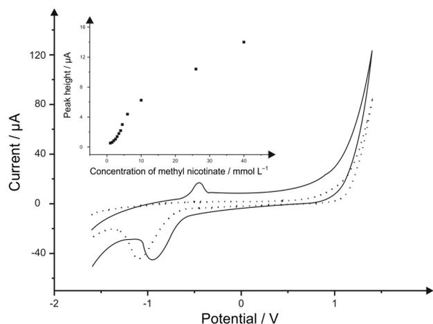
**Figure 2.** Typical cyclic voltammograms recorded in the absence (dotted line) and presence (solid line) of methyl nicotinate ( $25 \text{ mmol L}^{-1}$ ) in a pH 7 phosphate buffer solution using a screen-printed electrode. Scan rate:  $100 \text{ mV s}^{-1}$  (vs. Ag/AgCl). Inset: A typical corresponding calibration plot result from additions over the range 1 to  $40 \text{ mmol L}^{-1}$ .
