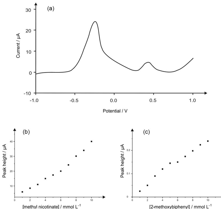
**Figure 4.** (a) A typical SWV recorded in a pH 7.4 phosphate buffer solution containing 4  $\text{mmol L}^{-1}$  methyl nicotinate (ca.  $-0.25$  V) and 4  $\text{mmol L}^{-1}$  2-methoxybiphenyl (ca.  $+0.4$  V). SWV parameters: frequency 20 Hz, scan potential 10 mV and amplitude 30 mV; (b) and (c) depict calibrations plots for the simultaneous additions of methyl nicotinate and 2-methoxybiphenyl respectively over the concentration range of 1 to 10  $\text{mmol L}^{-1}$ .
