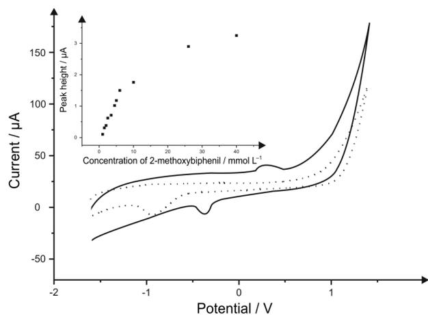
**Figure 3.** Typical cyclic voltammograms recorded in the absence (dotted line) and presence (solid line) of 2-methoxybiphenyl ( $40 \text{ mmol L}^{-1}$ ) in a pH 7 phosphate buffer solution using a screen-printed electrode. Scan rate:  $100 \text{ mV s}^{-1}$  (vs. Ag/AgCl). Inset: a typical corresponding calibration plot result from additions over the range 1 to  $40 \text{ mmol L}^{-1}$ .
