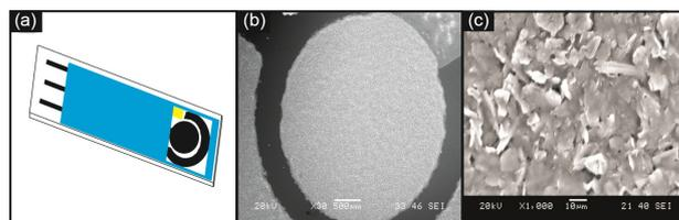
**Figure 1.** (a) Schematic diagram and (b) and (c) SEM images at increasing magnifications of a graphite screen-printed sensor (SPE).
