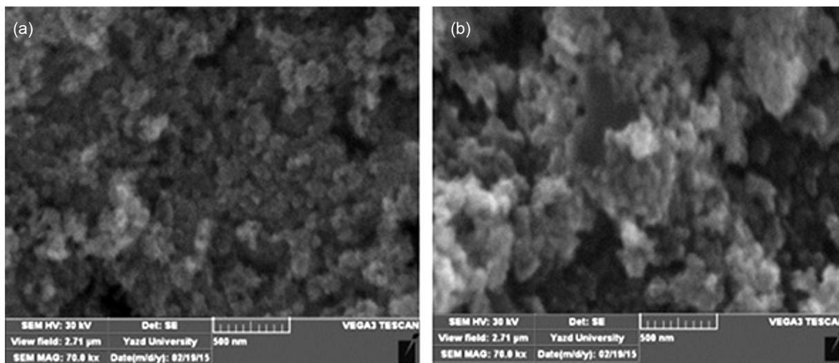
**Figure 3.** SEM image of (a) MNPs; (b) IL modified MNPs.
