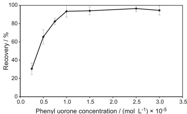
**Figure 5.** Effect of phenylfluorone concentration on extraction of Cr<sup>VI</sup>. Conditions: pH = 5; sample volume, 40 mL; amount of sorbent, 15 mg; extraction time, 15.0 min; stirring rate, 1000 rpm; eluent concentration, 2.0 mol L<sup>-1</sup>; eluent volume, 350  $\mu$ L and amount of Cr<sup>VI</sup>, 12 ng.
