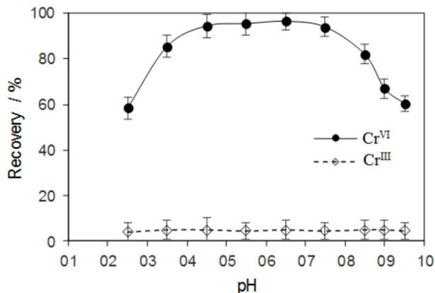
**Figure 4.** Effect of sample pH on the extraction of Cr<sup>VI</sup>. Conditions: sample volume, 40 mL; phenylfluorone concentration,  $2.5 \times 10^{-5}$  mol L<sup>-1</sup>; amount of sorbent, 15 mg; extraction time, 15.0 min; stirring rate, 1000 rpm; eluent concentration, 2.0 mol L<sup>-1</sup>; eluent volume, 350  $\mu$ L and amount of Cr<sup>VI</sup>, 12 ng.
