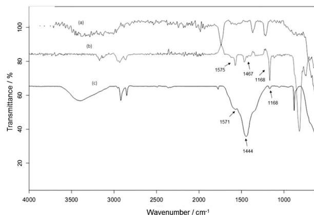
**Figure 2.** FTIR spectra of (a) MNPs; (b) ionic liquid; (c) MNPs coated with IL.
