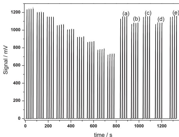
**Figure 7.** Records of the luminometer readout. From left folic acid standard solution  $0.0, 0.1, 0.2, 0.5, 0.7, 1.0, 1.3, 1.7$  and  $2.0 \text{ mg mL}^{-1}$ ; followed of five folic acid samples.
