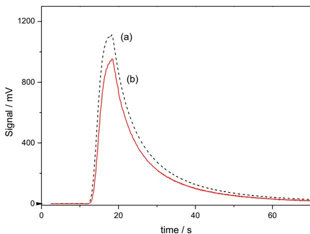
**Figure 3.** Records of the luminometer readout. Curves (a) and (b) are signals generated using a blank solution and a  $0.6 \text{ mg mL}^{-1}$  folic acid solution, respectively.
