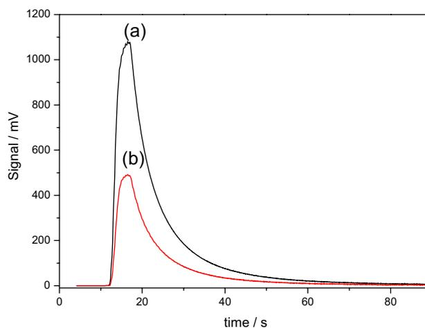
**Figure 6.** Effect related to the use of two photodiodes. Records (a) and (b) correspond to the measurements carried out using two and only one photodiode, respectively.
