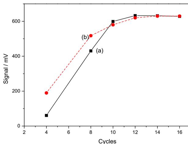
**Figure 4.** Effect of the sampling cycles. Curves (a) and (b) correspond to the variation of sample and luminol solution inserting cycles, respectively, achieved using a  $1.0 \text{ mmol L}^{-1}$  luminol solution prepared in a  $0.4 \text{ mol L}^{-1}$  NaOH medium and a  $20 \text{ mmol L}^{-1}$  hexacyanoferrate(III) solution.
