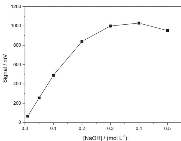
**Figure 5.** Effect of the sodium hydroxide concentration. Results obtained processing a blank solution. Other parameters as described in the previous sections.
