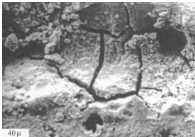
Figure 6. A scanning electron microscopy image of the interior of the crevice of a sample submitted to discontinuous voltammetry, and held at +5300mV for 120 min.
