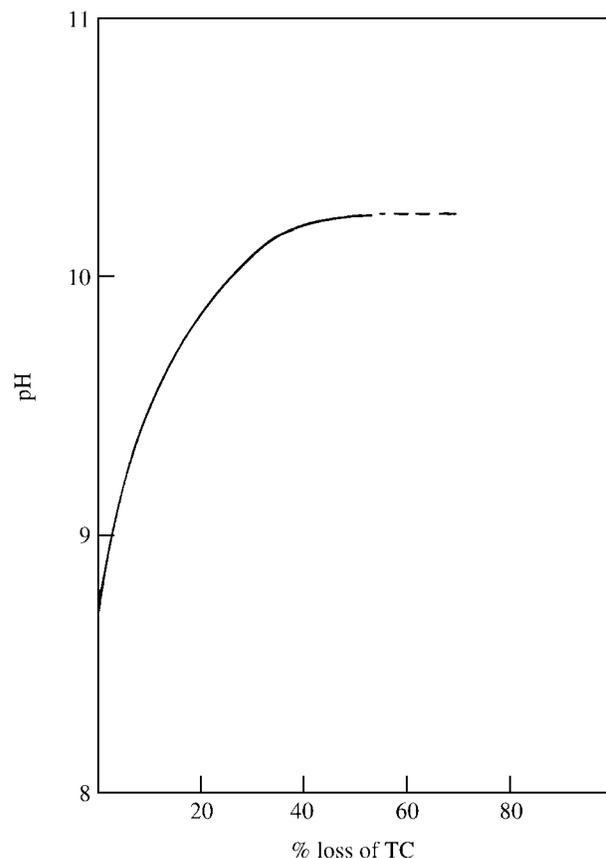
**Figure 2.** The effect of loss of  $\text{CO}_2$  on the pH of the solution. Starting from a 0.2 M sodium bicarbonate solution, the curve shows the changing pH as function of the percentage of removed TC.
