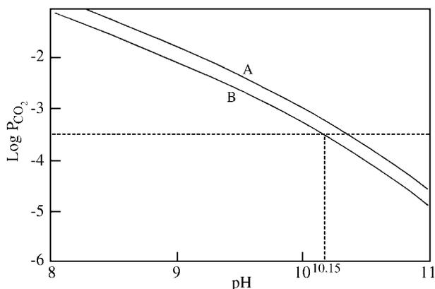
**Figure 1.**  $P_{\text{CO}_2}$  [atm] of sodium bicarbonate solutions as function of the pH. A: 0.2 M TC, B: 0.1 M. Broken line:  $\text{CO}_2$  partial pressure of the atmosphere. Solution B is in equilibrium with the atmosphere at pH 10.15.
