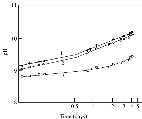
**Figure 4.** Semi-log plot of the data of Fig. 3 demonstrating that the evasion process is still going on after 11 days.
