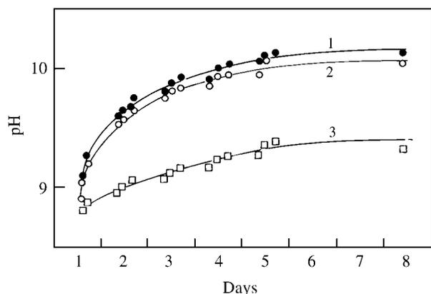
**Figure 3.** Removal of TC by various processes and the resulting changes of pH. Curve 1: fast loss of CO<sub>2</sub> in an air-mixed solution. Curve 2: same as 1, but with an algae culture. Its liberation of CO<sub>2</sub> from respiration keeps the curve below curve 1. Curve 3: slow evasion of CO<sub>2</sub> from a medium stirred without braking the water/air interface.
