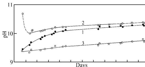
**Figure 5.** All curves represent cultures with algae. 1 and 2: air-mixed, 3 stirred without braking the interface. The pH of experiment 2 was initially raised by adding NaOH to a pH above the equilibrium value. Note that curves 1 and 2 approach asymptotically each other. Curve 3 shows again the slow evasion of CO<sub>2</sub> from a solution, when the interface is kept stable.
